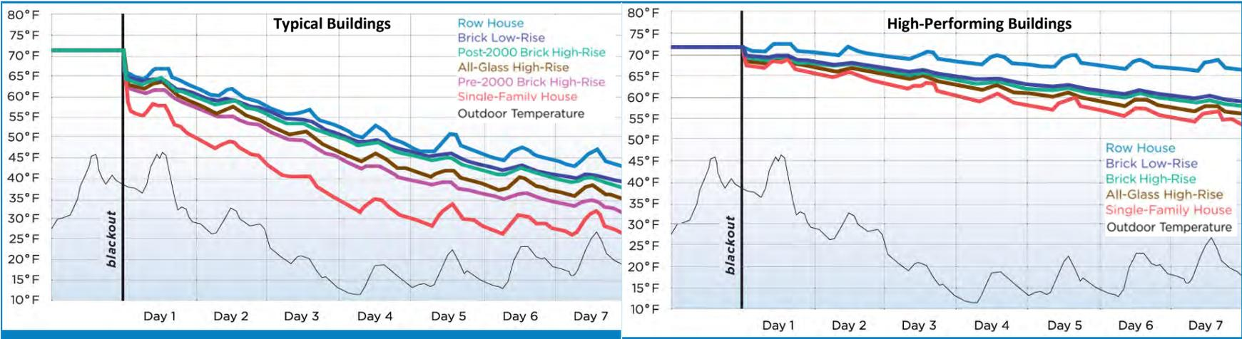
**Figure 21** ■ Modeled indoor temperatures for typical and high-performing buildings during an extended summer power outage (Urban Green Council, 2014).
